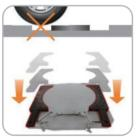
There are rubber pads on the turntable to make sure the tires are in a stable plane
