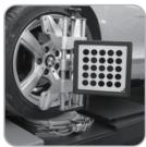
• There is no electronic components and sensors on the target board
