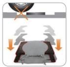
There are rubber pads on the turntable to make sure the tires are in a stable plane
