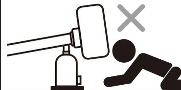
4. After use, turn the release valve slowly counterclockwise to lower the vehicle onto the ground. (Do not get under or let anyone else under the vehicle while lowering.)
