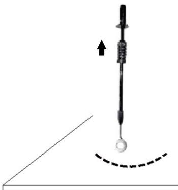
Remove the welding gun, pull out the round washer with a heavy hammer
