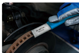
Scrape off rust.
