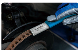
Scrape off rust.
