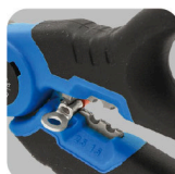
• Crimping terminal of cable
