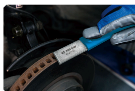
Scrape off rust.
