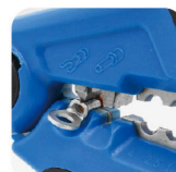
• Crimping terminal of cable
