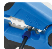
• Crimping terminal of cable
