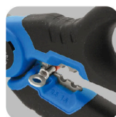
• Crimping terminal of cable
