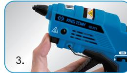
3. Press the ignition button and wait 2-3 min (Make sure the indicator on)
