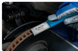
Scrape off rust.
