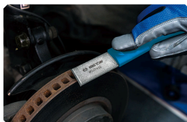
Scrape off rust.
