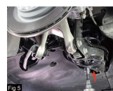
Fig 5 Use an air impact wrench to compress the spring
