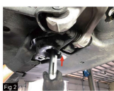
Fig 2 Insert the main tool body into the spring
