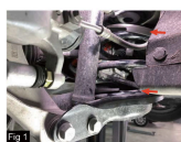
Fig 1 Place upper and lower discs on spring
