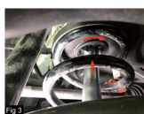
Fig 3 Insert through the disc and make a half turn to connect the tool and disc
