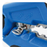
• Crimping terminal of cable
