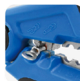
• Crimping terminal of cable
